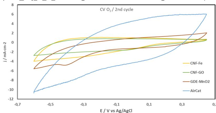
Figure 8. Cyclic voltammetry (CV) of material for air-cathode electrode.
