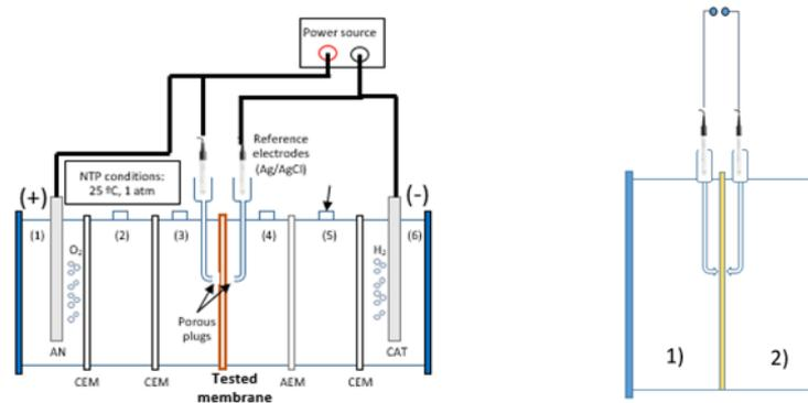
Figure 3. Electrical resistivity cell (left), Permselectivity cell (right)
