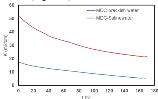
Figure 9. Desalination of saline (35 gNaCl/L) and brackish (10 gNaCl/L) water using an air-cathode MDC.
