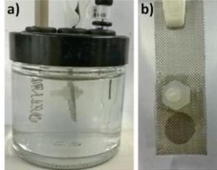
Figure 5. a) Three electrodes abiotic electrochemical cell and b) 6 mm circle metal doped carbon fiber membrane.
