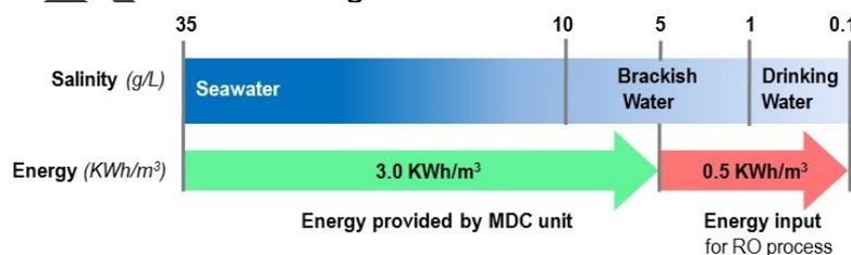
Figure 1. Energy concept for MDC coupled with RO.
