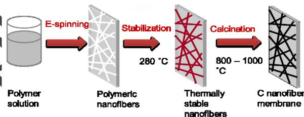
Figure 4. Metal doped carbon nanofiber fabrication process through electrospinning.
