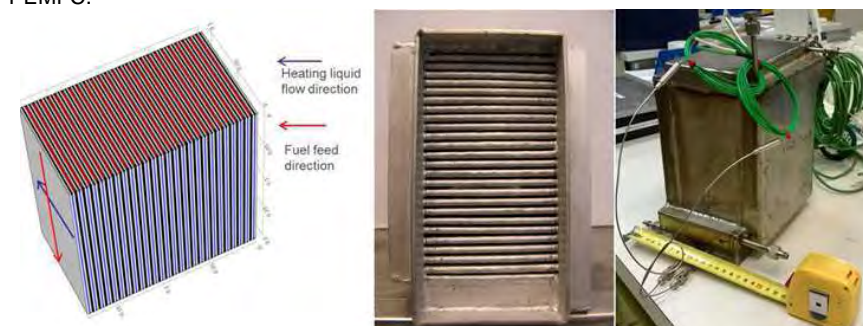
Figure 1. The structure of the LT-MSR. To the left: flow directions of the reformer. To the middle: the physical appearance of the catalyst layers. To the right: the finalized reformer.
